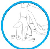
Unscrew the screw and remove the axle
