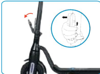
Pull the handle safety up, then lower the handle and fold the scooter mast back onto the platform.
