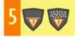
Protection against physical contact with dangerous elements - wire Protection against dust (sand, road dust
